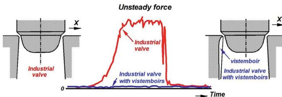
Figure 5. Influence of vistemboirs on the unsteady forces in an existing industrial valve
