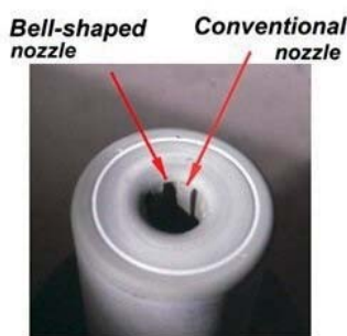
Figure 3. Valve provided with vistemboirs (kinetic energy degraders) : The ventose valve
